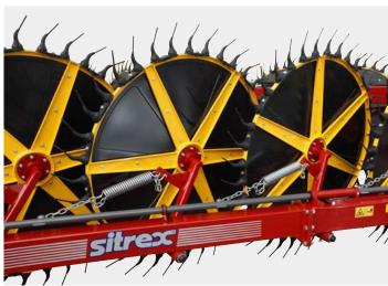
**All MKE-PRO rakes feature 60" raking wheels with 18 double tines (36 tines) of ø 0.276"**. The wheel frame is extremely stiff for a perfect collection of wet, green, heavy and voluminous hay. Windbreaks are standard on all models for an easy and quick formation of smooth, uniform windrows.
